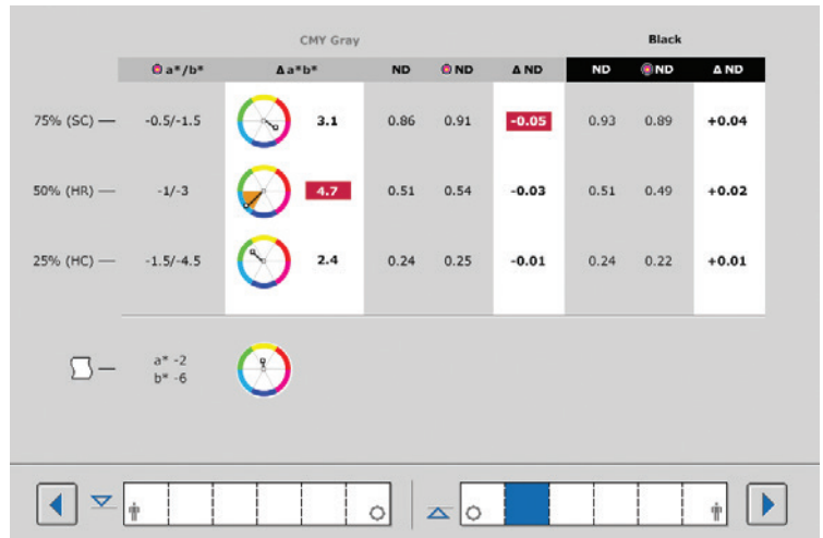
During the print run, operators can view live performance reporting that tracks G7 conformance through CMY gray balance and tonality values.
